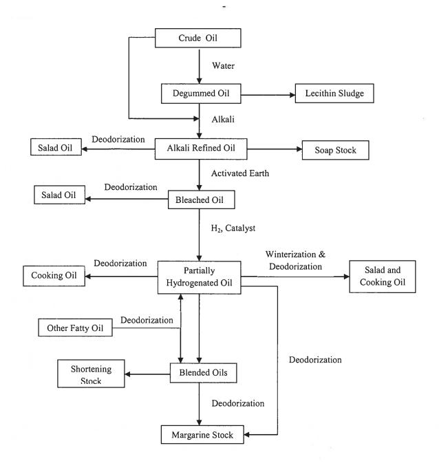
Figure 2. Basic oil refinement flowchart.6
