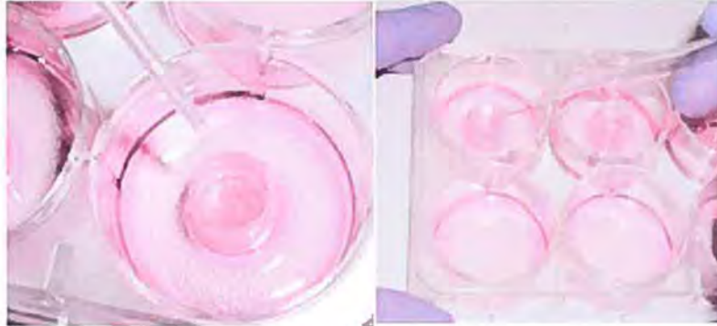
Figure 5: Application of semisolids (positive displacement pipette - detail) and subsequent spreading using bulb headed Pasteur pipette
