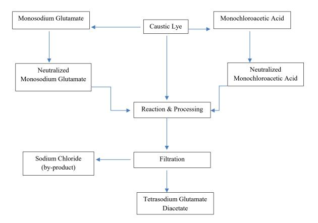
Figure 2. Manufacturing flow chart of a Tetrasodium Glutamate Diacetate tradename product.9
