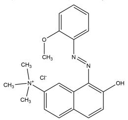
Figure 1. The azo dye, Basic Red 76
